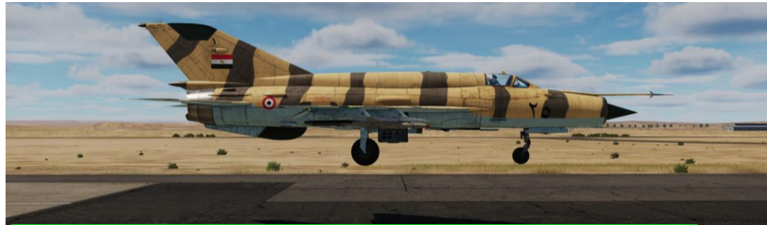
Good touchdown: fast and low Angle of Attack (0-10 deg) – very gentle contact with the ground
