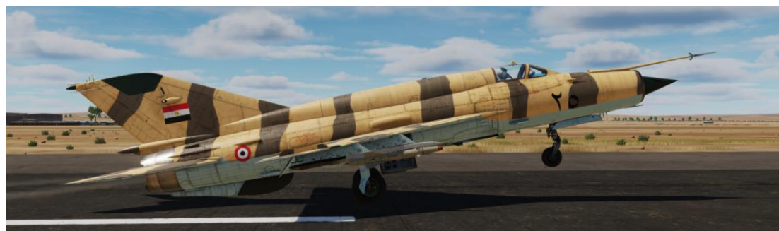
Bad touchdown: slow and high Angle of Attack (20 deg). You are likely to violently smack your tail on the ground.
