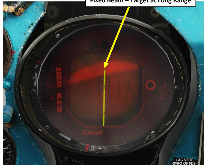
Fixed Beam – Target at Long Range
