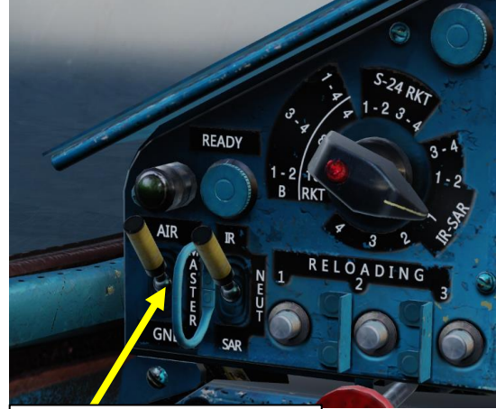
ASP-PFD Sight Master Mode Air/Ground Switch • UP: Air Mode • DOWN: Ground Mode
