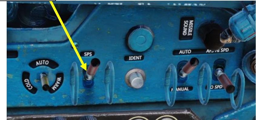
SPS (Flaps Boundary Layer Control System) Switch • UP: AUTO • DOWN: MANUAL
