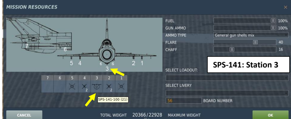
ASO-2 Countermeasure Cartridge Dispensers (Typical: 40 flares + 16 chaff)
