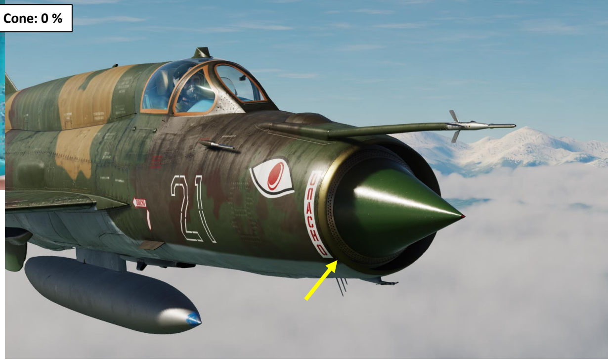
Nose Cone: 100 % - High Risk of Compressor Stall, AVOID!
